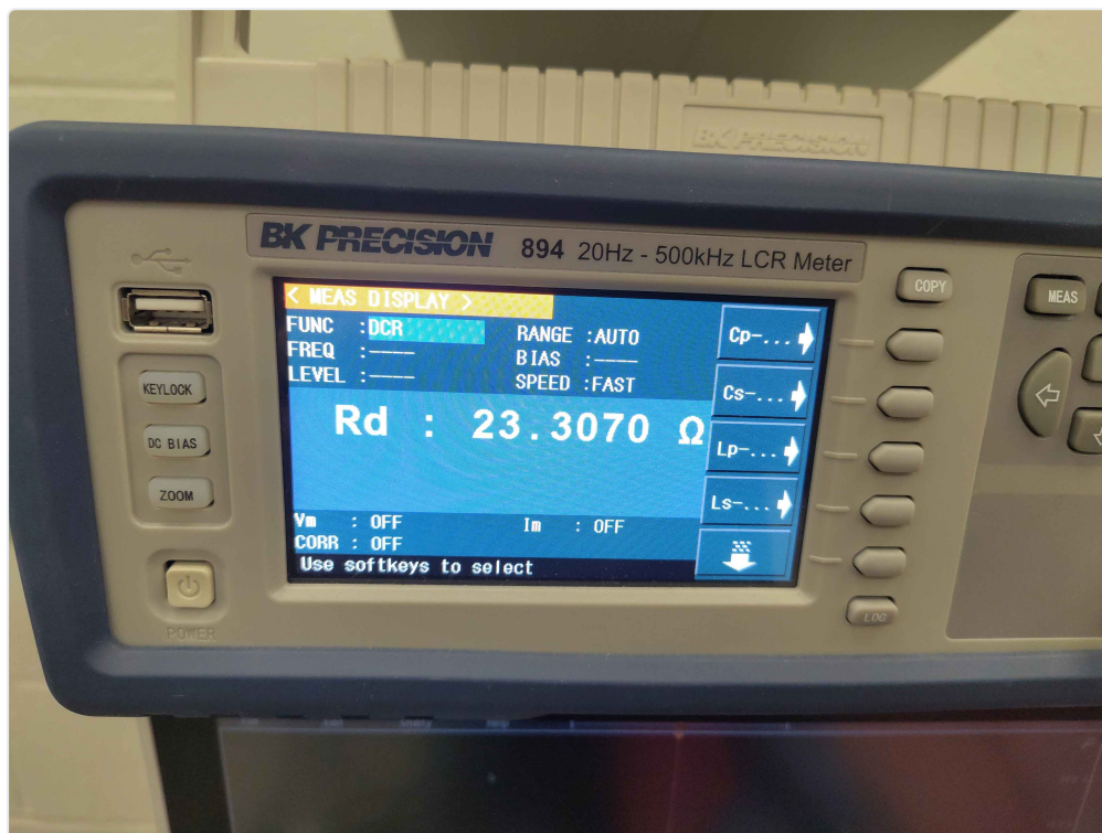
LCR meter DCR reading: R_d = 23.3070 \Omega
