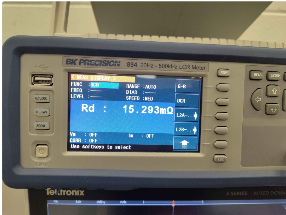
LCR meter DCR reading: R_d = 15.293 \text{ m}\Omega
