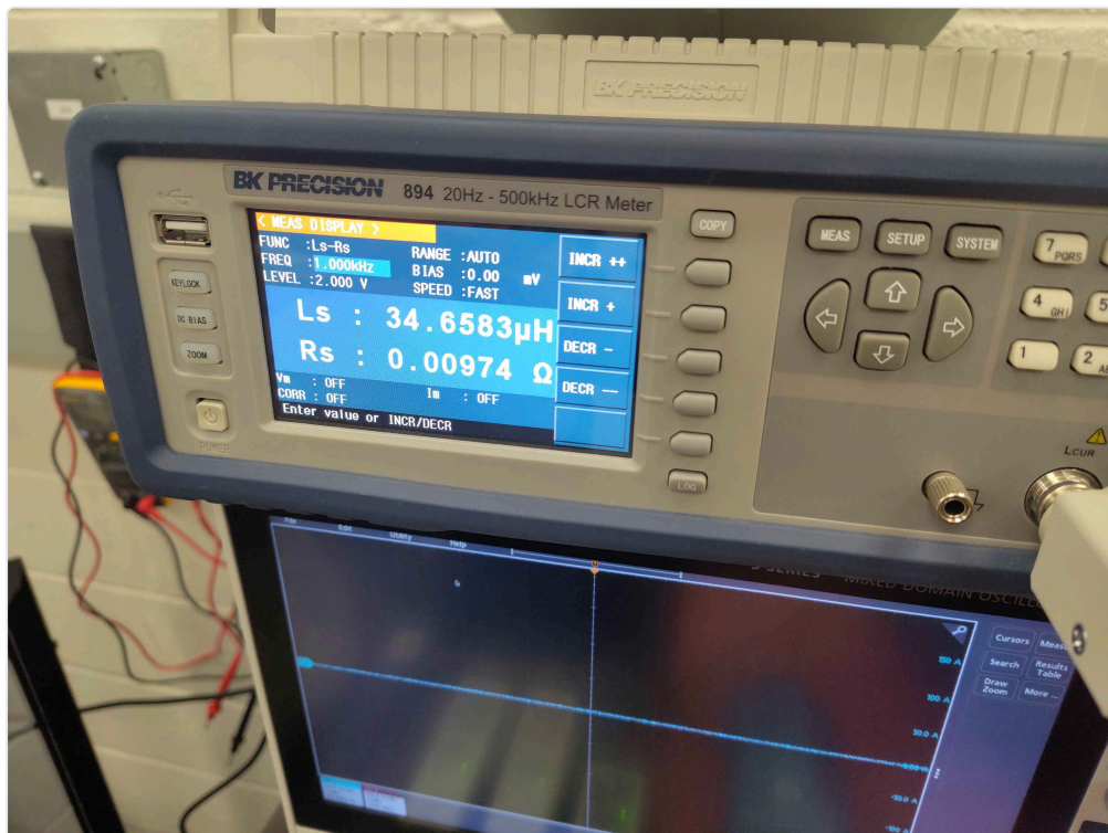
LCR meter Ls-Rs reading 2: L_s = 34.6583 \mu\text{H} , R_s = 0.00974 \Omega
