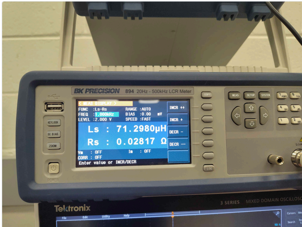
LCR meter Ls-Rs reading 1: L_s = 71.2980 \mu\text{H} , R_s = 0.02817 \Omega
