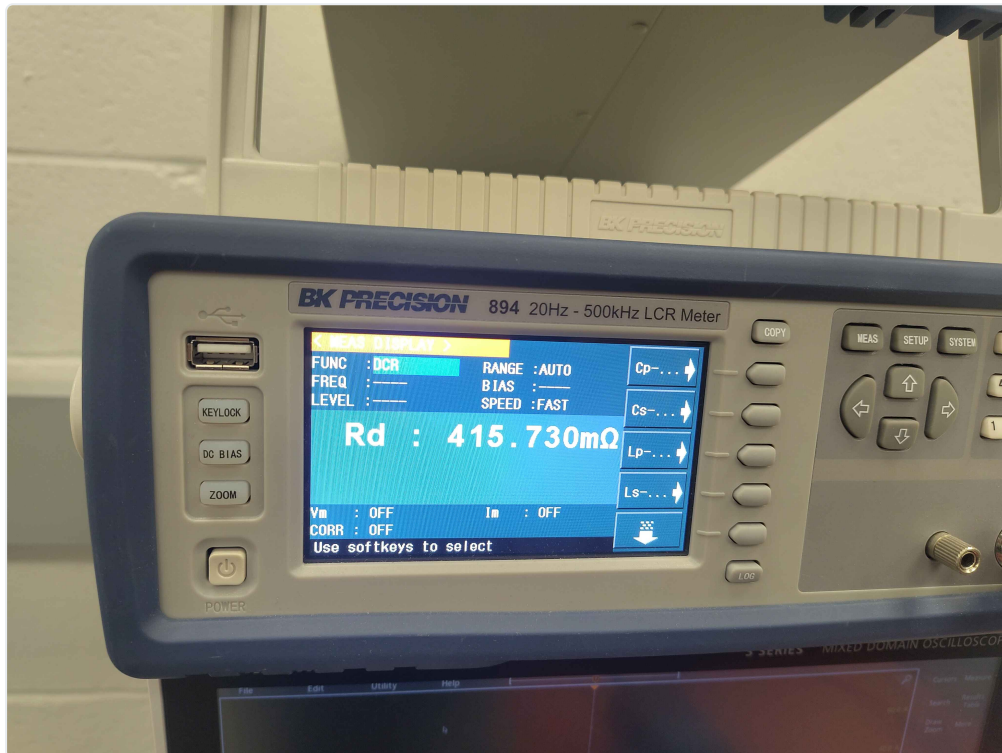
LCR meter DCR reading: R_d = 415.730 \text{ m}\Omega
