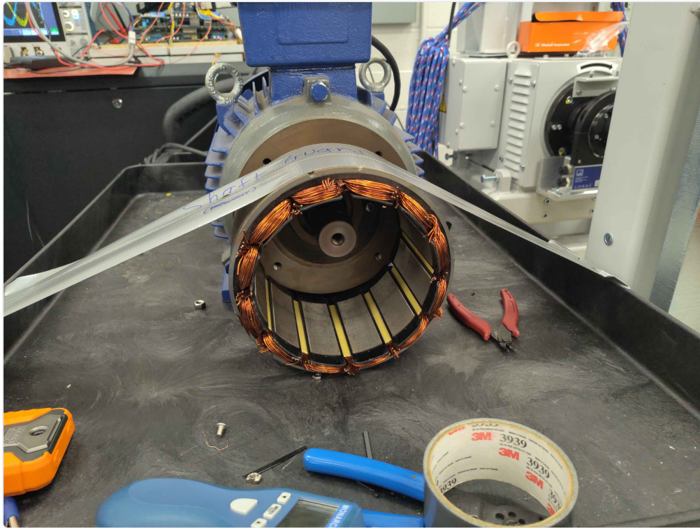
Induction motor stator windings prior to the run
