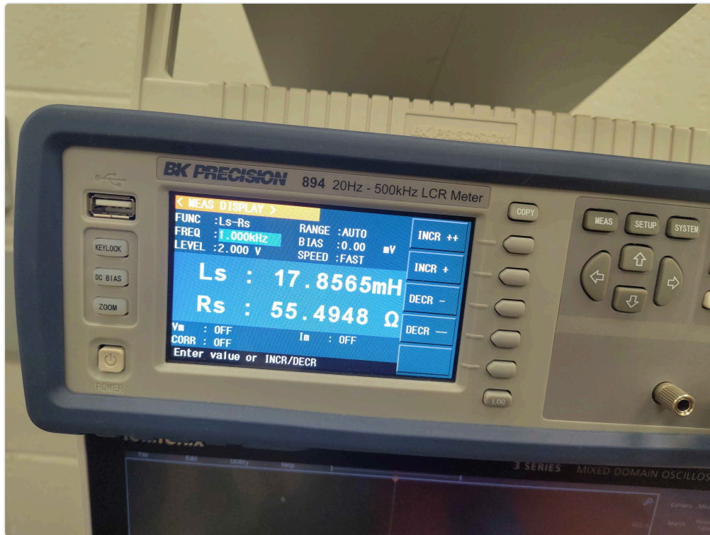
LCR meter Ls-Rs reading: Ls = 17.8565 mH, Rs = 55.4948 \Omega
