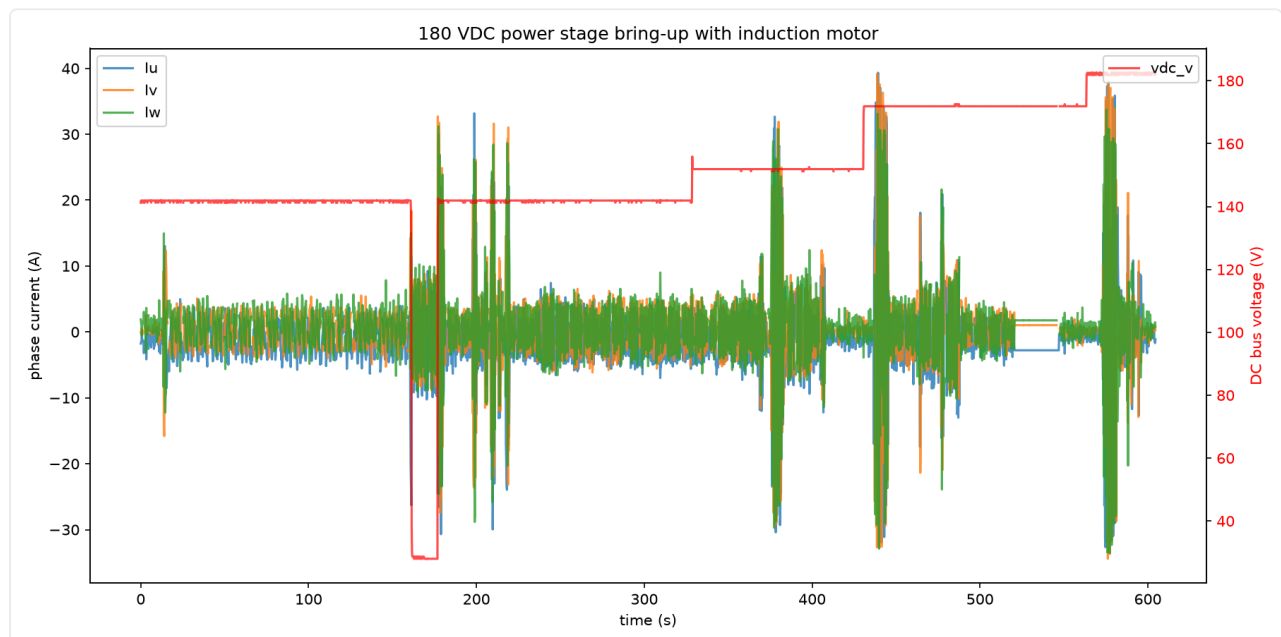
Telemetry overview of the 180 V bring-up: phase currents and DC bus voltage
