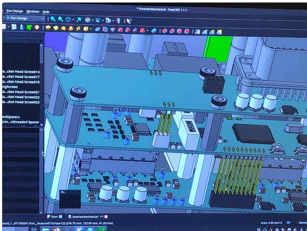
Checking connector placement and orientation against the CAD model
