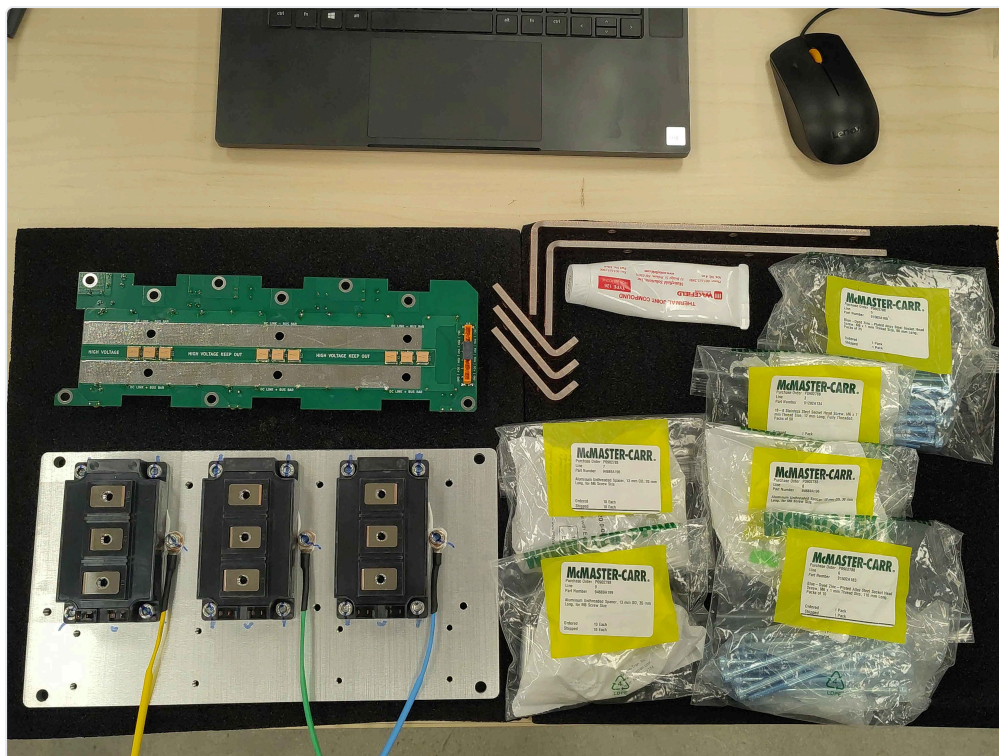
Overview of the workspace with heatspreader, spacers, bus bars, and filter board
