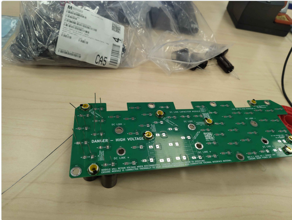
Soldering the standoffs to the mounting pads
