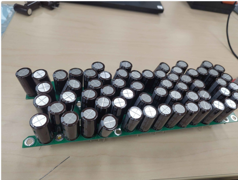
All 60 capacitors inserted on the component side of the board
