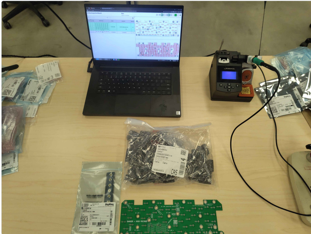
Workspace with PCB, capacitor reel, standoffs, soldering station, and BOM on a laptop
