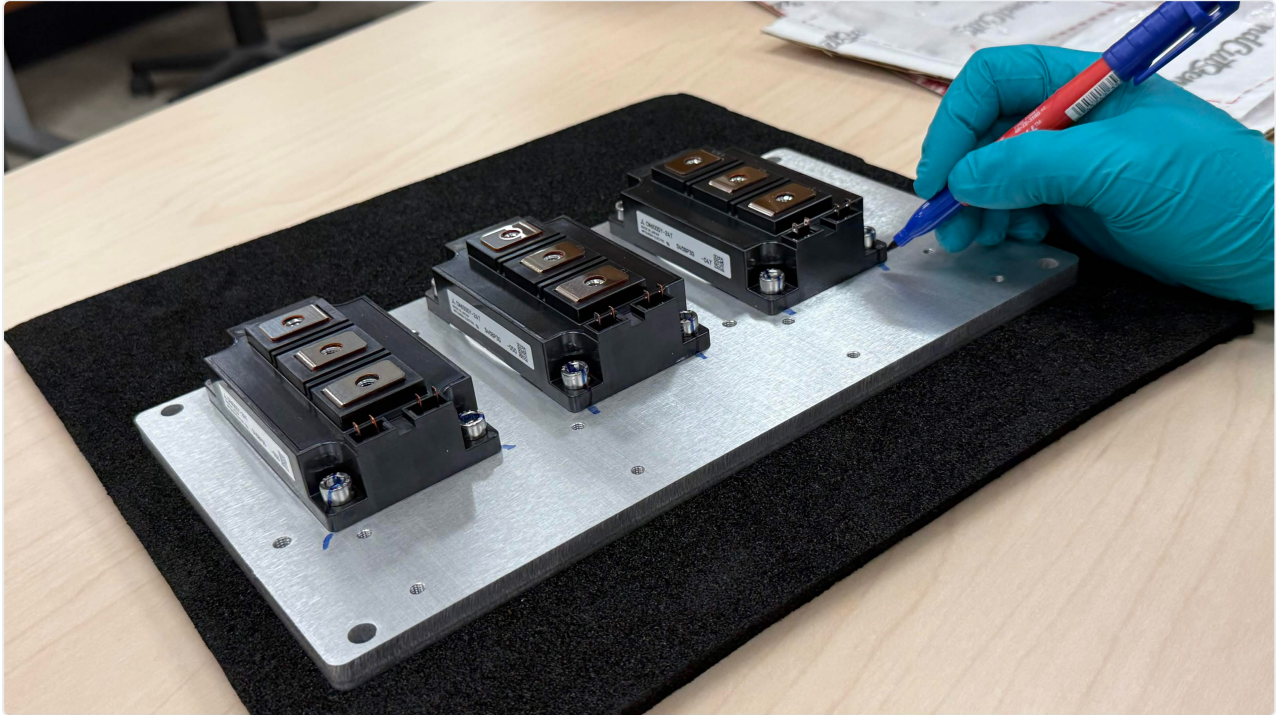
Applying a torque-strip mark from the screw head to the baseplate
