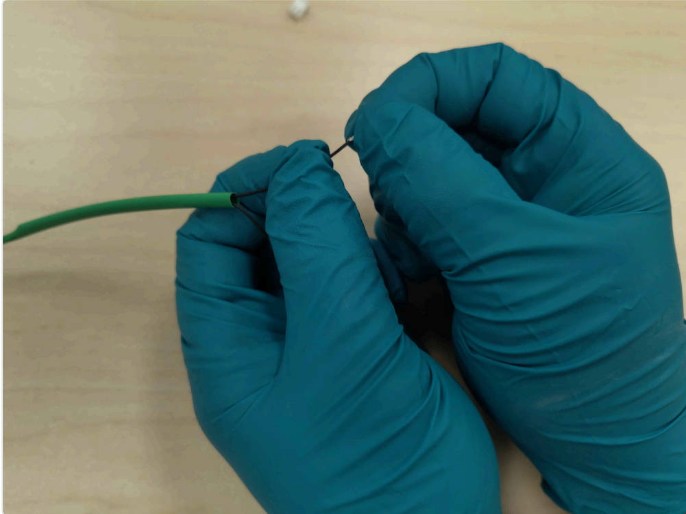
Performing a pull test on a freshly crimped terminal
