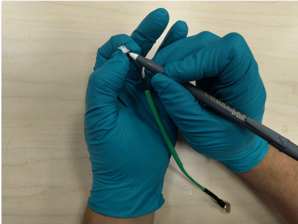
Inserting a crimped terminal into the housing
