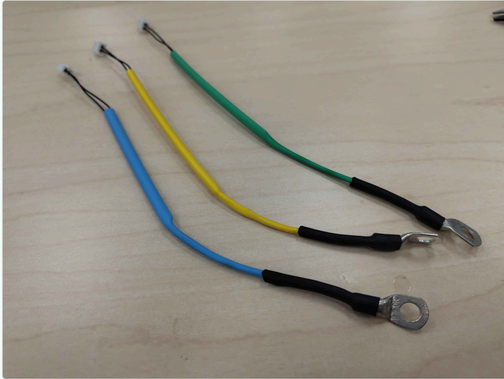
Three finished harnesses with yellow, green, and blue heat-shrink for phases U, V, and W
