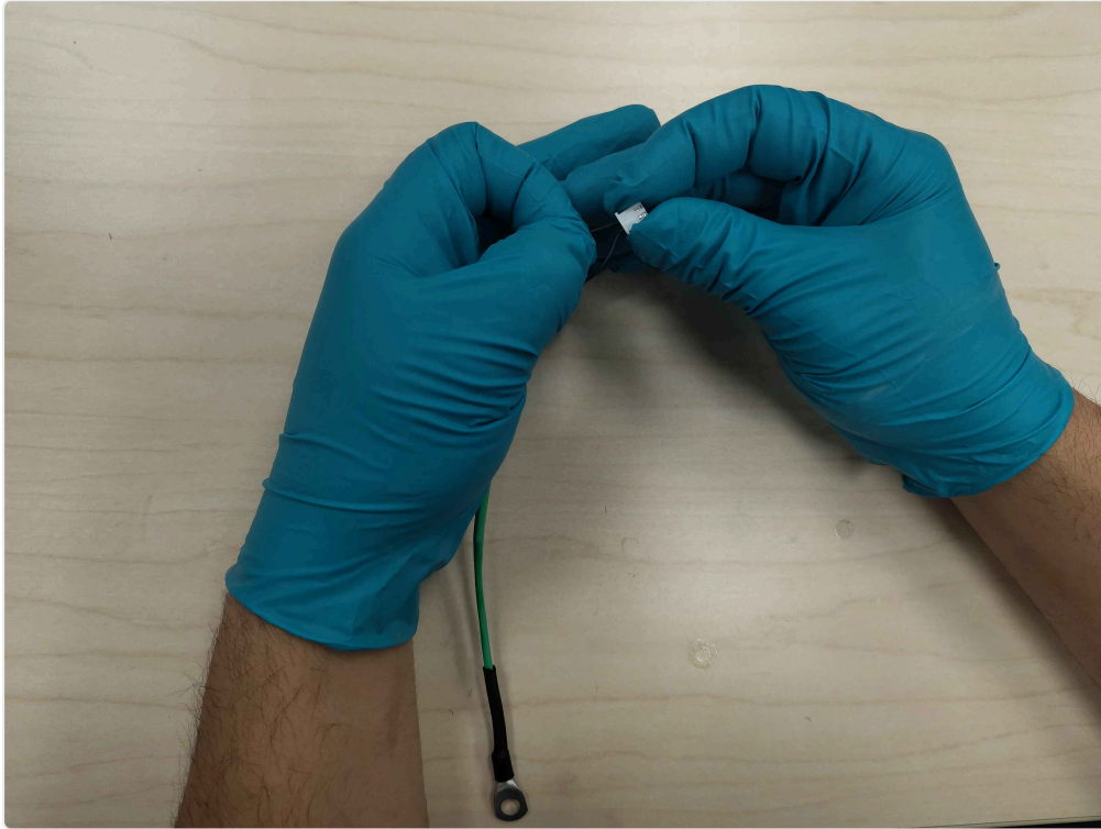
Pull-testing the wires after insertion to verify the locking tang
