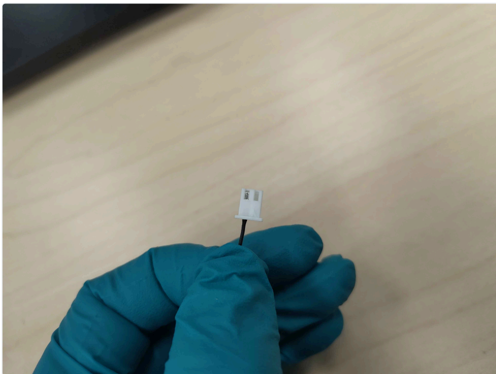
Terminal fully seated in the housing
