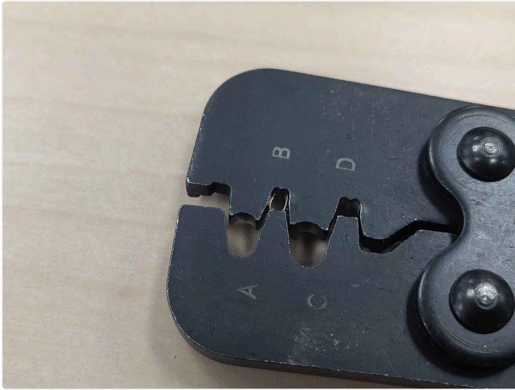
Terminal positioned in the crimping tool
