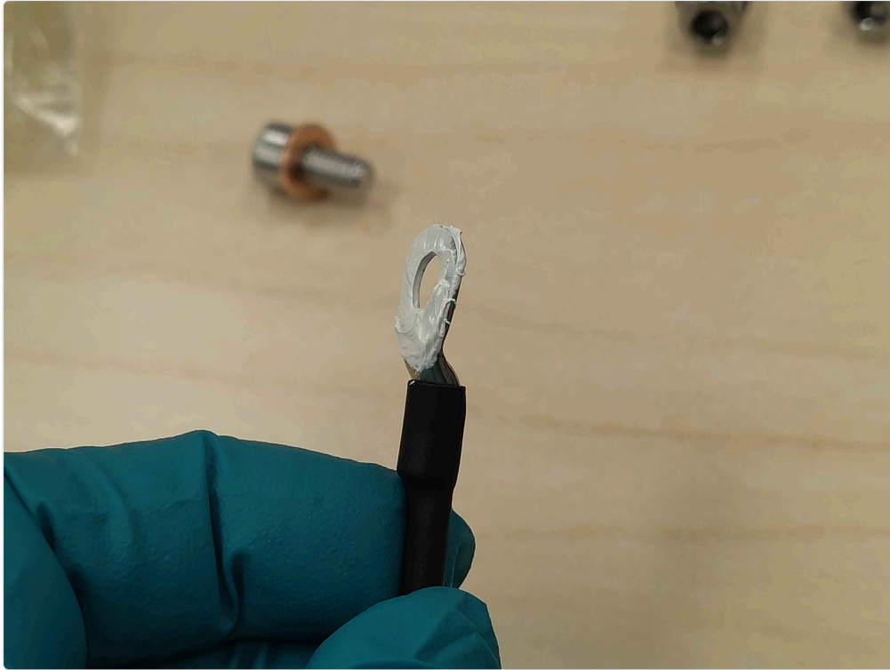
Thermal paste spread evenly across the lug contact surface
