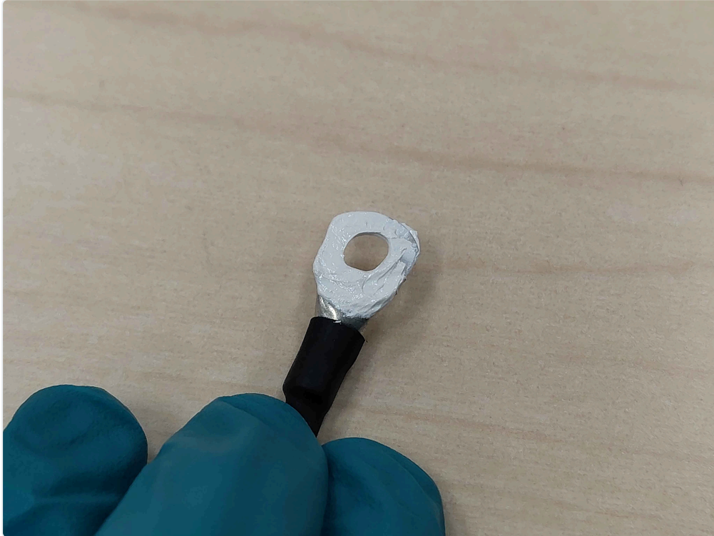
Thermal paste being applied to the underside of the ring lug
